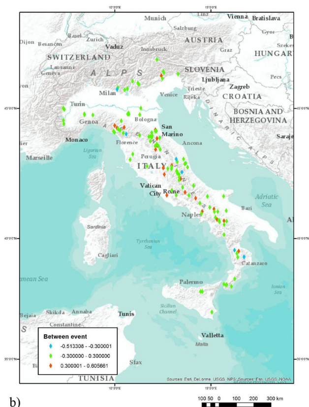
Fig. 13 Type 1 model Log-Lin 10 : a Between-event residuals versus magnitude M_w of the calibration earthquakes; b Spatial distribution of the calibration earthquakes; c Within-event residuals versus epicentral distance
