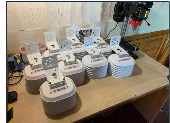
Example: atmospheric pressure sensors, Resolution 0.14 hPa, memory 21,700 data
